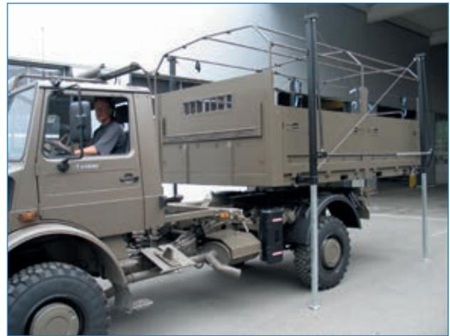
Type 297/B depositing system for changing modules on a vehicle.
