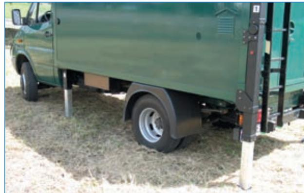
Type 287/B levelling support with automatic levelling mechanism.
