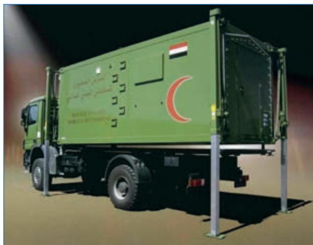
Type 260 lifting device with mobile surgical unit.
