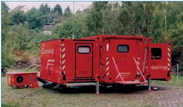
Type 260 lifting system with push out boom for fire brigade coordinating centre.
