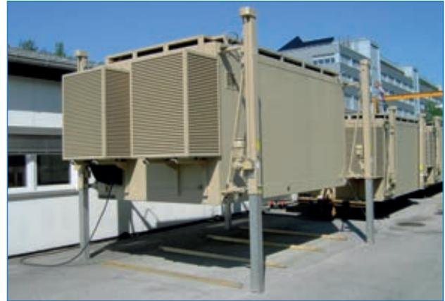
Type 260 lifting system with automatic position control.
